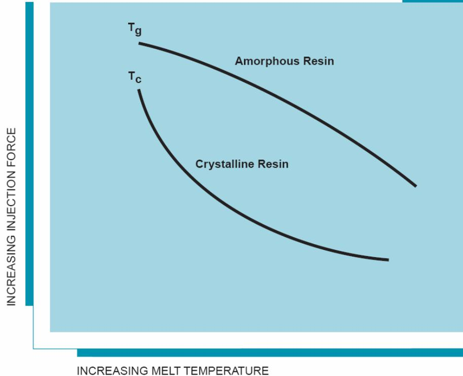
The force required to generate flow in a mold diminishes slowly above the glass transition temperature ( $T_g$ ) in amorphous thermoplastics, but drops quickly above the crystalline melt temperature ( $T_c$ ) in crystalline resins.
